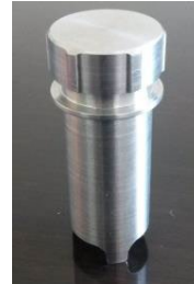
1) Metal tube (7mL) designed using inox steel
