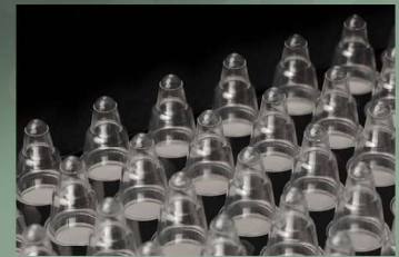
Extreme close up (with the plate flipped) to show the bottom tips of the wells
