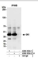
Detection of human and mouse QKI by western blot. Samples: Whole cell lysate from HeLa (15 and 50 μg), HEK293T (50μg), and mouse NIH 3T3 (50μg) cells. Antibodies: Affinity purified rabbit anti-QKI antibody A300-183A (lot A300-183A-2) used for WB at 0.04 μg/ml. Detection: Chemiluminescence with an exposure time of 3 minutes.
