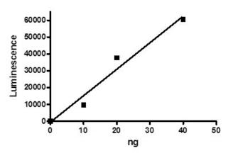
MLL1 complex enzyme activity, measured using the *MLL1 Complex Chemiluminescent Assay Kit*, BPS Bioscience #53008. Luminescence was measured using a Bio-Tek fluorescent microplate reader. *Data shown is lot-specific. For lot-specific information, please contact BPS Bioscience, Inc. at info@bpsbioscience.com*
