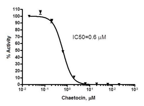
NSD2 enzyme activity, measured using the *NSD2 Chemiluminescent Assay Kit*, BPS Bioscience Catalog #53009. Luminescence was measured using a Bio-Tek fluorescent microplate reader. *Data shown is lot-specific. For lot-specific information, please contact BPS Bioscience, Inc. at <u>info@bpsbioscience.com</u>.*
