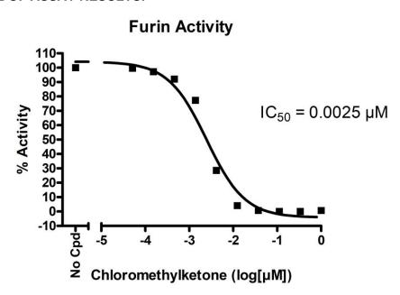
Inhibition of Furin enzyme activity by Chloromethylketone, measured using the Fluorogenic Furin Protease Assay Kit (BPS Bioscience #78040). Fluorescence intensity was measured using a Tecan fluorescent microplate reader. Data shown is lot-specific. For lot-specific information, please contact BPS Bioscience, Inc. at info @bpsbioscience.com
