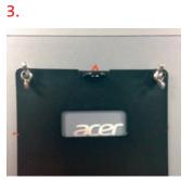
Remove the wing nuts from the back of the tablet.
