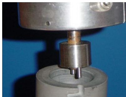
Figure 21. Coupling of motor and direct drive shaft
