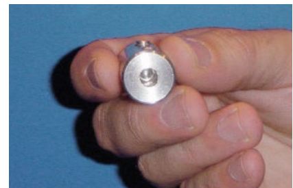
Figure 5. Coupling collar – smaller opening for drive shaft
