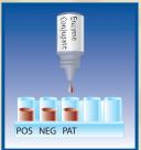
9 Add 2 drops of Enzyme Conjugate to all wells. Seal the plate and incubate for 30 minutes at room temperature.
