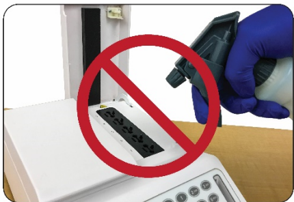
DO NOT spray the Alethia instrument directly with any solution
