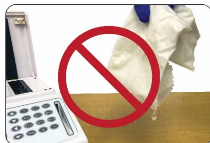
DO NOT use oversaturated cloths or oversaturated foam swabs for cleaning
