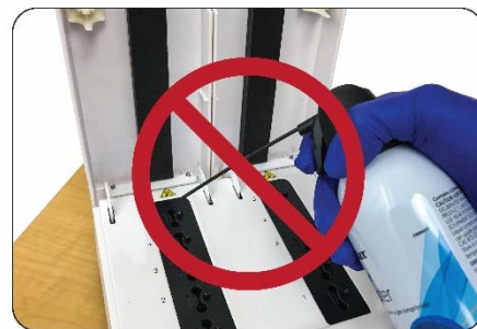
DO NOT attempt to clean the Alethia instrument using compressed air
