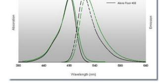
Comparison of fluorescence absorption and emission spectra for DyLight 488 and Alexa Fluor 488 in PBS, pH 7.2
