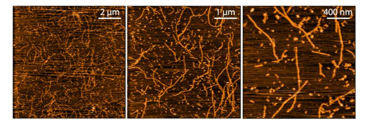
AFM of amyloid beta pyroglutamate 3-42 fibrils (catalog# SPR-492). Atomic force microscopy analysis of 1.0 mg/mL samples diluted to 0.1 mg/mL in 2% DMSO + 10 mM HCl, mounted on freshly cleaved mica, washed, dried and analyzed with tapping mode. Representative images are 10 x 10  $\mu$ m x-y (left) and 5 x 5  $\mu$ m x-y (middle) and 2 x 2  $\mu$ m x-y (right), all with a z-range of 6 nm.
