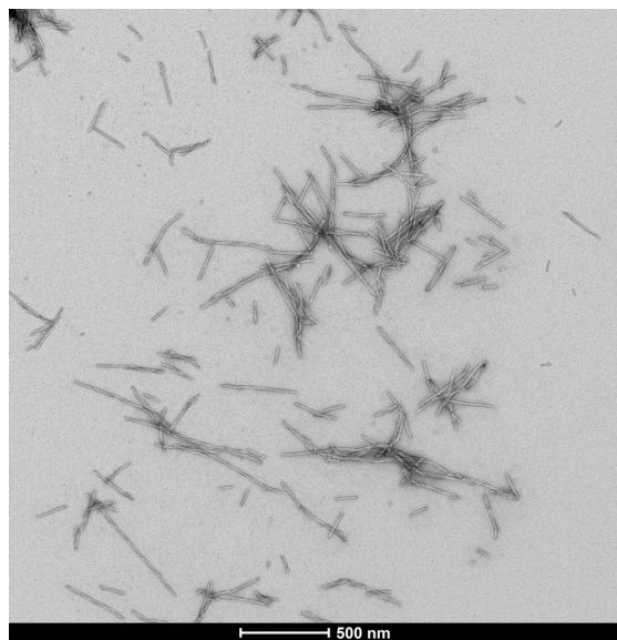
Representative TEM image of ATTO-488 conjugated Alpha Synuclein E114C Pre-Formed Fibrils (SPR-518-A88), 500nm scale. Negative stain transmission electron microscopy images of SPR-518 acquired at 80 Kv on carbon coated 400 mesh copper grids using phosphotungstic acid and uranyl acetate stain.
