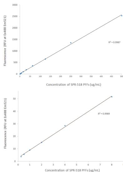
Fluorescent signal of alpha-synuclein E114C-ATTO-488 PFFs (SPR-518-A88). SPR-518 concentration and fluorescence (excitation 488nm, emission 521 nm) exhibit a linear relationship at all concentrations tested (250 ng/mL – 500 µg/mL).
