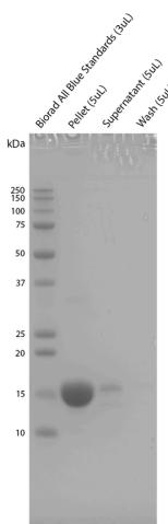
Sedimentation assay on ATTO-488 conjugated Alpha Synuclein E114C Pre-Formed Fibrils (SPR-518-A88). Samples were pelleted at 15,000 x g, washed, and then re-centrifuged. Fibril samples are prepared in denaturing conditions prior to running on the gel. SDS-PAGE analysis on a 12% Bis-Tris gel shows that the majority of fibril is insoluble.
