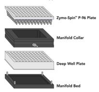
Diagram of the EZ-Vac 96 Vacuum Manifold setup with the ZymoPURE<sup>TM</sup> 96 Plasmid Miniprep Kit components. Refer to sections A, B, and C for the vacuum manifold and plate assembly necessary for lysate clearing, DNA binding and washing, and elution, respectively.
