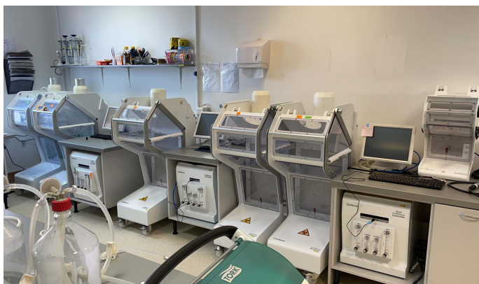
50L SU CellMaker bioreactors in a bacteriophage production lab
