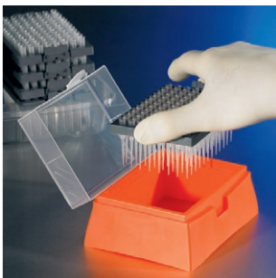
Insert deck into hinged rack.
