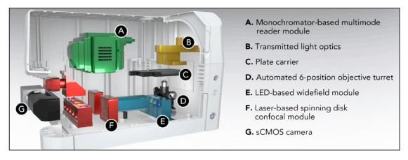
With a combination of spinning disk confocal and widefield imaging, plus multi-mode reader, Cytation C10 is truly ready for any assay. And since Cytation C10 is a modular, upgradable instrument, you can get the functionality you need today and add modules later as your needs expand.
