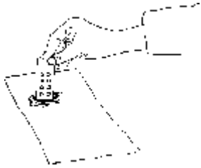
7. Blot edge of slide(s) on absorbent paper. next step
