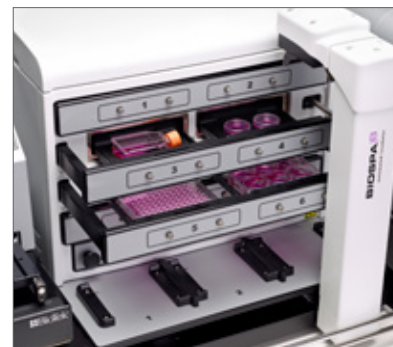
BioSpa 8 holds up to 8 microplates and other labware.
