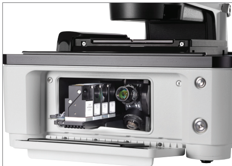
Easy access to filter/LED cubes and objectives.
